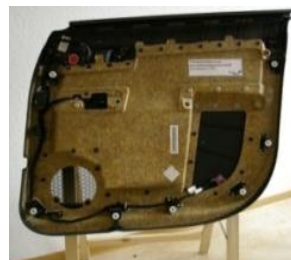
Fig. 2 Image of Hemp plastic interior of a car door, Courtesy: Wikipedia, Wikimedia
