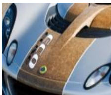
Fig. 4 Image of Hemp fiber automotive bonnet, Courtesy: Gardner Publications Inc.
