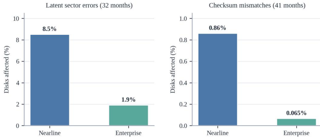
Fig. 2. Disk-level prevalence of latent errors and checksum mismatches.
